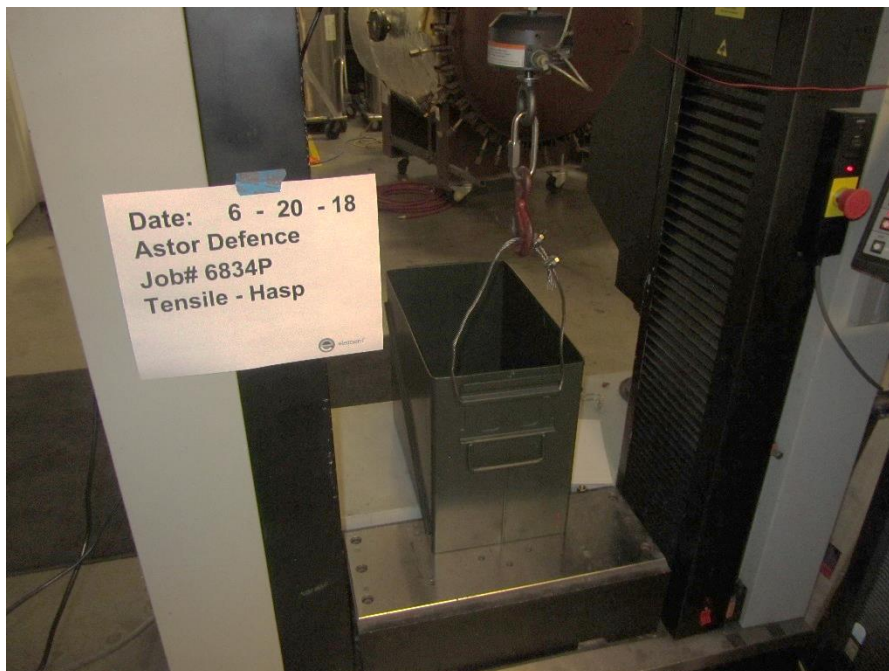
Photo 8 – Sample set up to begin testing
